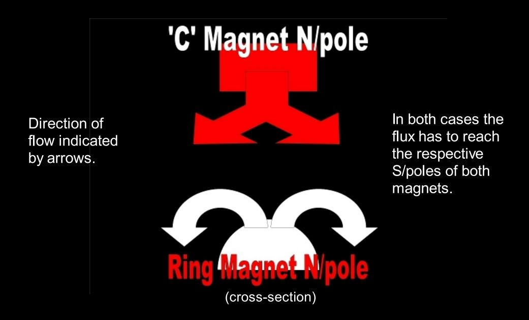
Here we are looking at the ring magnet in cross-section. Now we can see that – although the respective flux flows from both magnets originate from N/poles – both are travelling in the same direction.
