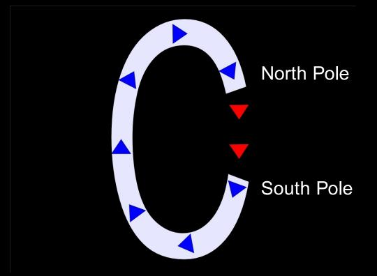
I've chosen this shape (**NB** which will be modified as we progress) for our third element: the 'C' magnet, because with it we can physically model the actual shape of the Earth's magnetic field - which is essentially the shape of a ring doughnut (tech speak: torus).
