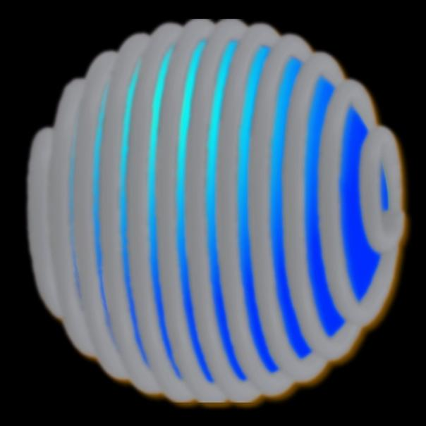
Here we see an electrical coil wound vertically around the electromagnetically transparent sphere.
