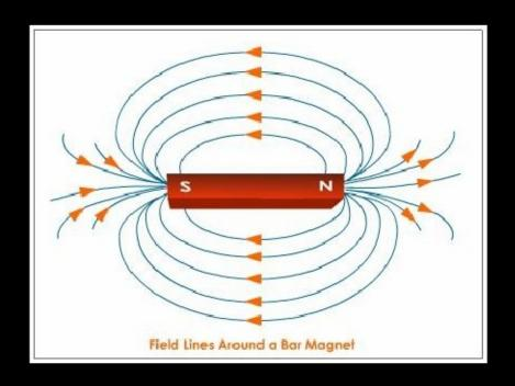
This image represents a simple bar magnet and the way in which the magnetic flux – represented by the flow lines – travels from the magnet's North Pole to it's South Pole. The direction of flow between the two poles is always the same. When travelling through the magnet the flow is South to North. When travelling around it – through the air – the direction is always North to South.
