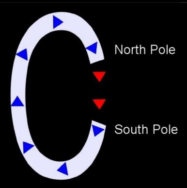
I've chosen this shape (**NB** which will be modified as we progress) for our third element: the 'C' magnet, because with it we can physically model the actual shape of the Earth's magnetic field - which is essentially the shape of a ring doughnut (tech speak: torus).
